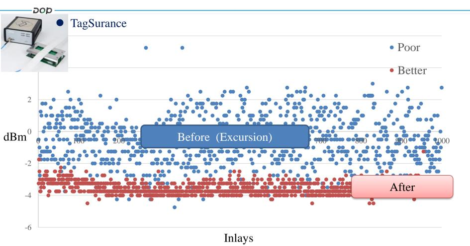
Improve mass production yield by stopping the IC Bonding machine as it is in a poor running condition.
