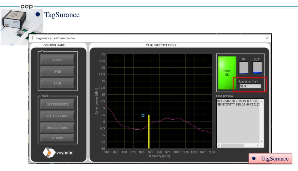
Faster measurement speed: It only takes 51.9ms for each tag to measure both TID and Sensitivity.
